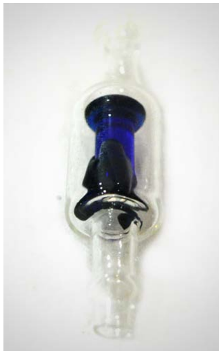
Figure 3: Check Valve Close-up
